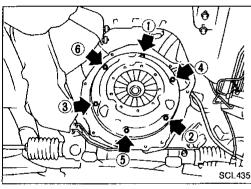
Tighten clutch cover fixing bolts in numerical order by 2 steps.
