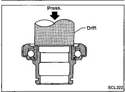
Install release bearing with suitable drift.
